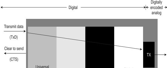
Going from the DTE device, the data is sent through the UART, which handles buffering and flow control with the host. The data compressor passes the data to the packetizer, which puts a checksum on it and sends it on to the DSP. The packetizer also handles retransmits if the data doesn't get through to the other DCE. The data travels onward to the digital to analog processor, which pushes the data out the RJ11 jack to the phone line. Receiving data goes in the reverse process.
