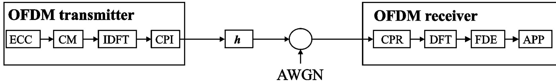
OFDM transmitter is a serially encoded system:
