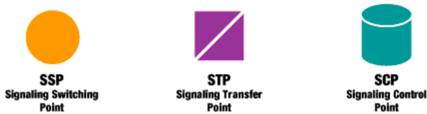
Figure 2. Signaling Network Elements
