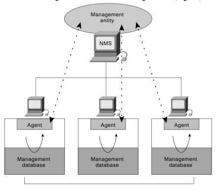
Figure 56-2 An SNMP-Managed Network Consists of Managed Devices, Agents, and NMSs
