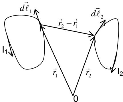
$$\vec{F}_2 = \frac{\nu_0}{4\pi} I_1 I_2 \oint_{\ell_1} \oint_{\ell_2} \frac{d\vec{\ell}_2 \times [d\vec{\ell}_1 \times (\vec{r}_2 - \vec{r}_1)]}{|\vec{r}_2 - \vec{r}_1|^3} = \oint_{\ell_2} I_2 d\vec{\ell}_2 \times \left\{ \frac{\nu_0}{4\pi} \oint_{\ell_1} I_1 d\vec{\ell}_1 \times (\vec{r}_2 - \vec{r}_1) \right\} = \oint_{\ell_2} I_2 d\vec{\ell}_2 \times \vec{B}(\vec{r}_2)$$
