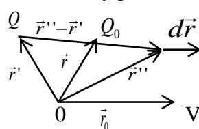
$$E_{pol}(\vec{r}) = \int_{\vec{r}}^{\vec{r}_0} \vec{F}(\vec{r}'') \cdot d\vec{r} + E_p(\vec{r}_0) = \int_{\vec{r}}^{\vec{r}_0} Q_0 \vec{E}(\vec{r}) d\vec{r} + E_p(\vec{r}_0) =$$
