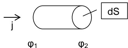
$$dI = \frac{\varphi_1 - \varphi_2}{R} = \frac{-(\varphi_2 - \varphi_1)}{R} = \frac{-d\varphi}{\frac{1}{\sigma} \cdot \frac{d\ell}{dS}} = \sigma \frac{dS}{d\ell} \cdot (-d\varphi)$$
