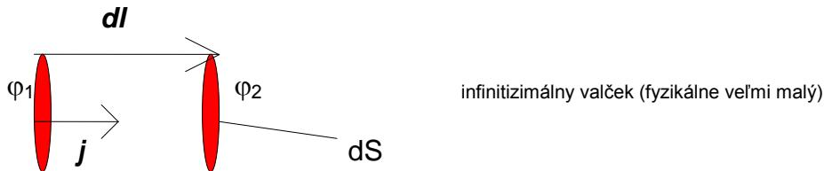
$$dI = \frac{\varphi_1 - \varphi_2}{R} = -\frac{(\varphi_2 - \varphi_1)}{R} = \frac{-d\varphi}{\frac{1}{\sigma} \frac{dl}{dS}} = \sigma \frac{dS}{dl} (-d\varphi)$$
