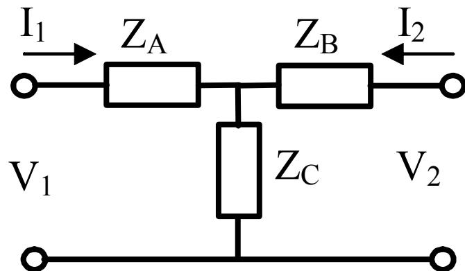
$$I_2 = 0 \quad \left\{ \begin{array}{l} Z_{11} = \frac{V_1}{I_1} \Big|_{I_2=0} = Z_A + Z_C \\ Z_{21} = \frac{V_2}{I_1} \Big|_{I_2=0} = Z_C \end{array} \right.$$
