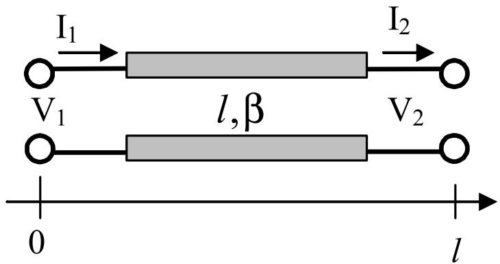
$$\left\{ \begin{array}{l} V_1 = V^+ + V^- , \quad I_1 = \frac{1}{Z_0} (V^+ - V^-) \\ V_2 = V^+ e^{-j\beta l} + V^- e^{j\beta l} \\ I_2 = \frac{1}{Z_0} (V^+ e^{-j\beta l} - V^- e^{j\beta l}) \end{array} \right.$$
