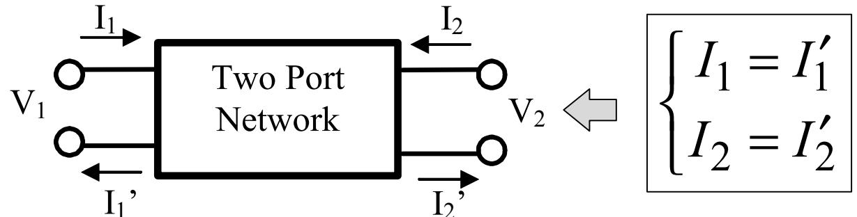
$$\begin{aligned} V_1 &= Z_{11} \cdot I_1 + Z_{12} \cdot I_2 \\ V_2 &= Z_{21} \cdot I_1 + Z_{22} \cdot I_2 \end{aligned}$$
