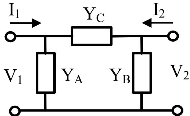
$$V_2 = 0 \rightarrow \left\{ \begin{array}{l} Y_{11} = \frac{I_1}{V_1} \Big|_{V_2=0} = Y_A + Y_C \\ Y_{21} = \frac{I_2}{V_1} \Big|_{V_2=0} = -Y_C \end{array} \right.$$
